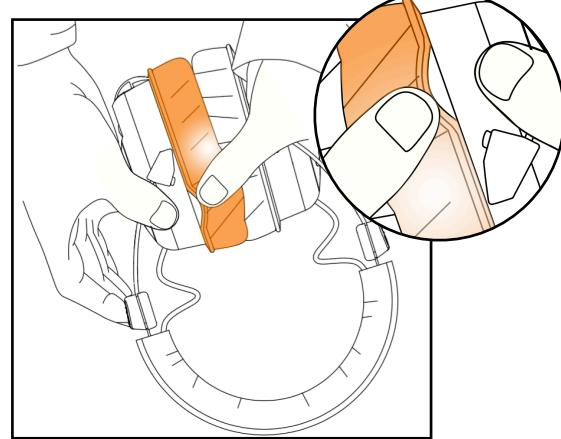
You can take off the head band cushions for cleaning or replace with new one. Hold the edge of the cushion and pull from the first button.
