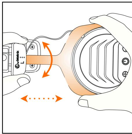
Before wearing the Wire-Free Pro headphones for the first time you should adjust it properly to achieve the best sound and ambient noise attenuation. A proper way of wearing will reduce the fatigue of your ear. As shown in the figure : Pull or push to select the appropriate lock-in position on both sides of the headphones folk. The dot will help you memorize the position for next time adjustment. The ear pads will tilt automatically according to your head size.
